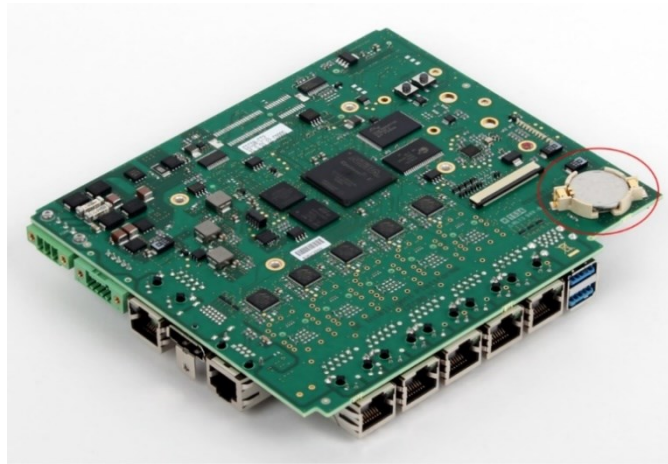
Figure 5: Location of RTC Battery on CPE400/CPL410
