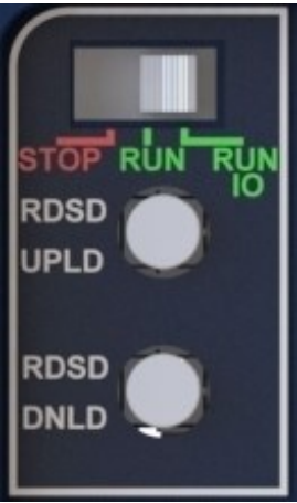
Figure 9: CPE330 Run/Stop Switch and RDSD Switches
